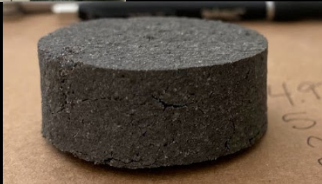
CSM-LHT-1G post-sintering Diameter: ~5.01cm Height: ~2.10cm
