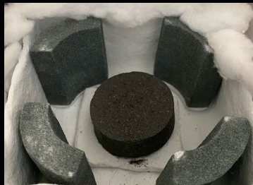
CSM-LHT-1G post-sintering Diameter: ~5.01cm Height: ~2.10cm
