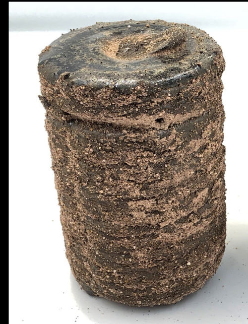
Sample of laser melted CSM-LHT-1 simulant, 1.3kg (size of a soda can)
