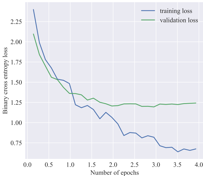
Fig. 6. Learning curves of training and validation loss during custom named-entity recognition model training.
