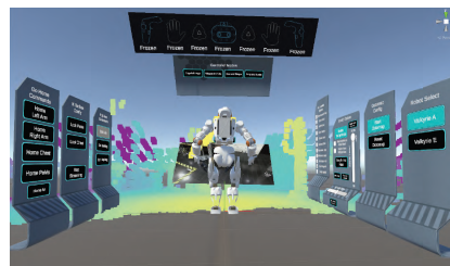
(b) NASA’s VR interface. Menus surround the operator to control Valkyrie and enable shared autonomy tools. Robot state, data visualizations, and augmented reality views are displayed.
