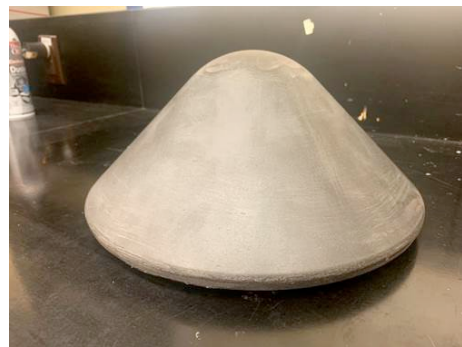
11" capsule with AMTPS heat shield flown by Univ. of Kentucky on NG-16
