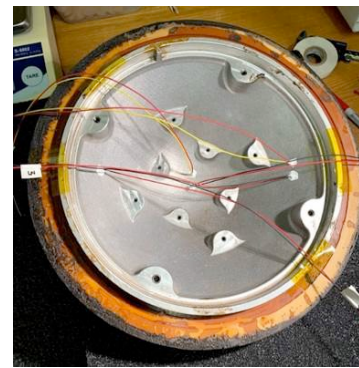
11" capsule with AMTPS heat shield flown by Univ. of Kentucky on NG-16
