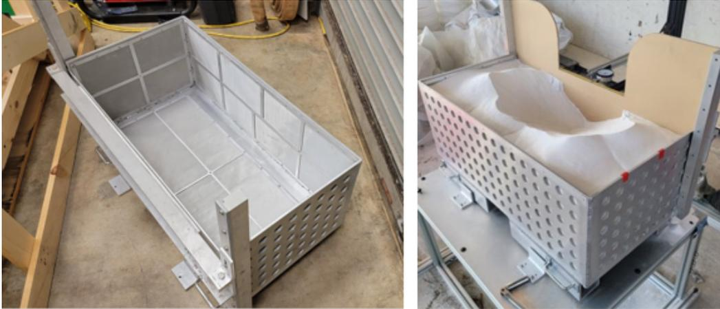
Figure 8. [left] Empty regolith simulant test bin demonstrating the wire mesh interior wall design to prevent particles spilling through the gas escape holes. [right] Testing of the bin with silica sand and a dummy splitter plate.
