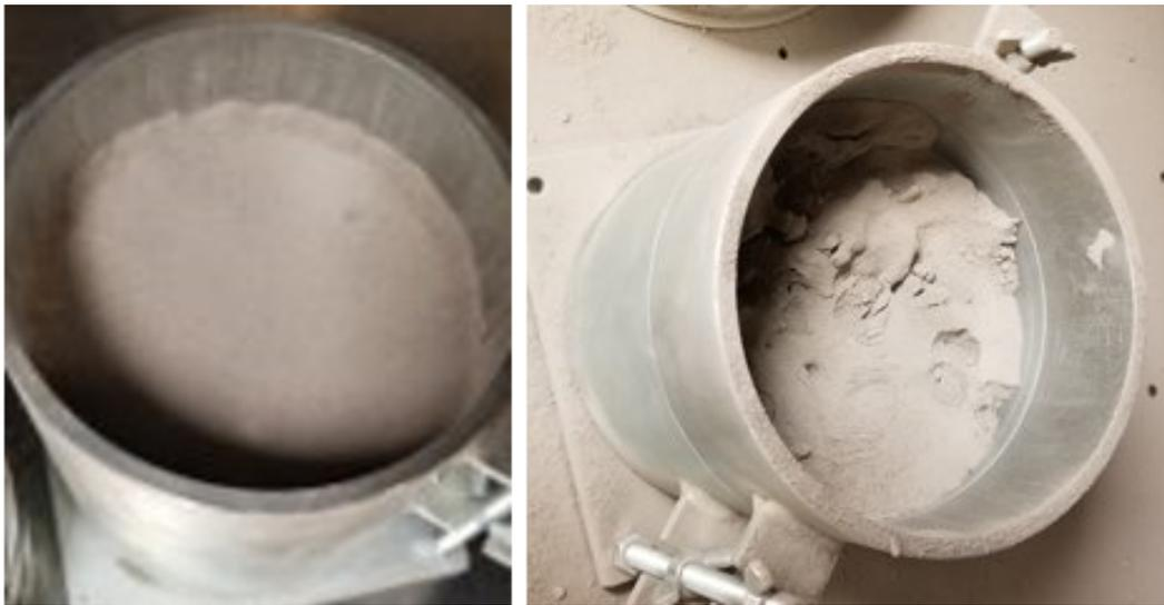
Figure 3. [left] BP-1 regolith simulant before vacuum pump-down. [right] BP-1 after pump-down. The surface of the simulant has been significantly altered due to vacuum eruptions.
