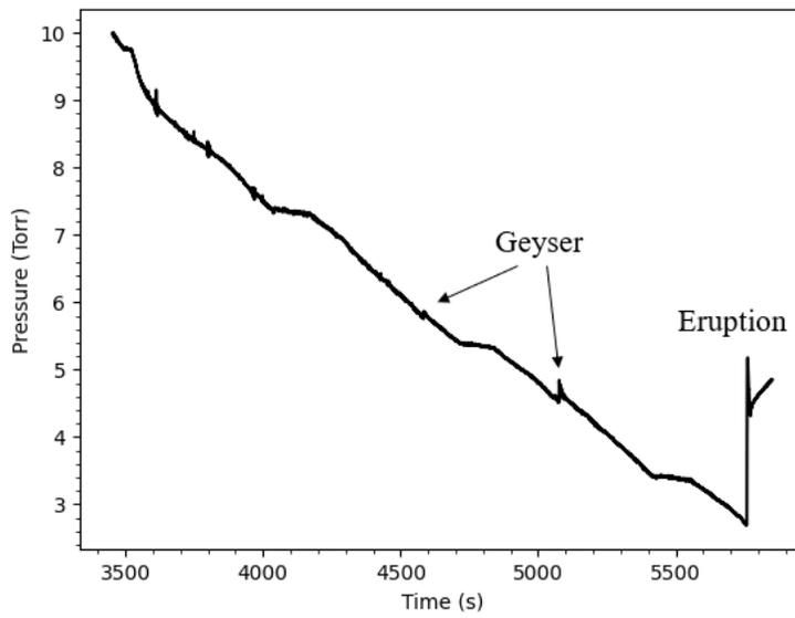
Figure 7. Pump down of undried BP-1 in a one-gallon soil mold. The rate was  $\sim 0.2$  Torr/min. The small spikes in pressure indicate micro-eruptions, or geysers, that are not visibly noticeable. Large spikes in pressure indicate a vacuum eruption that results in a visible change in the regolith simulant bed.
