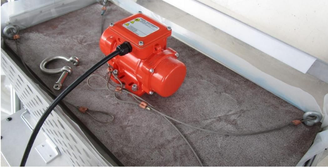
Figure 5. Top plate vibration setup for regolith simulant compaction testing.
