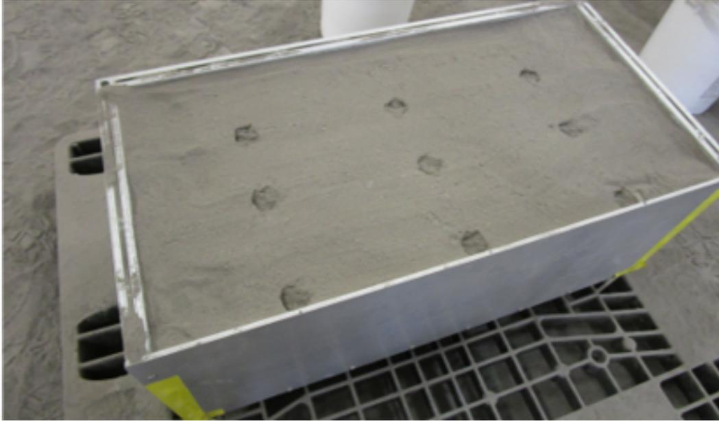
Figure 4. Shear vane testing locations for geotechnical characterizations.
