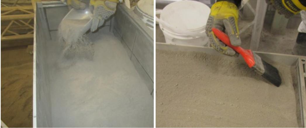
Figure 6. [left] “Snowing” technique for producing most consistent geotechnical characterizations, and [right] using a paint brush to level the surface.
