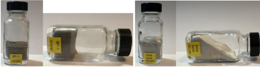
Figure 2. Comparing the behavior of regolith simulants. [left] BP-1. [right] Silica sand. In both cases the samples were lightly compacted by tapping prior to being laid flat. The interlocking (or bridging) behavior of course BP-1 is demonstrated.
