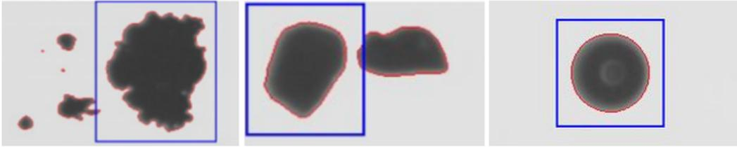
Figure 1. Comparison Fine Particle Analyzer images of three example regolith simulants. [left] Irregularly shaped coarse BP-1. [middle] Relatively smooth silica sand. [right] Spherical glass beads.
