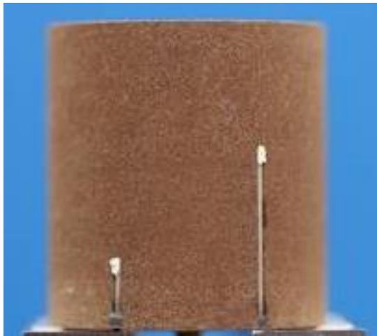
Artemis 1 & 2 Thermal Plugs with embedded Thermocouples
