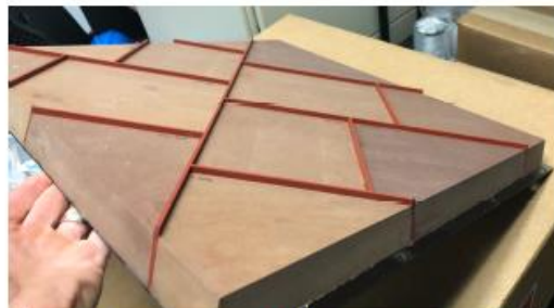
Heat Shield Avcoat Block/Seam Array in Combined Convective/Radiant Heating
