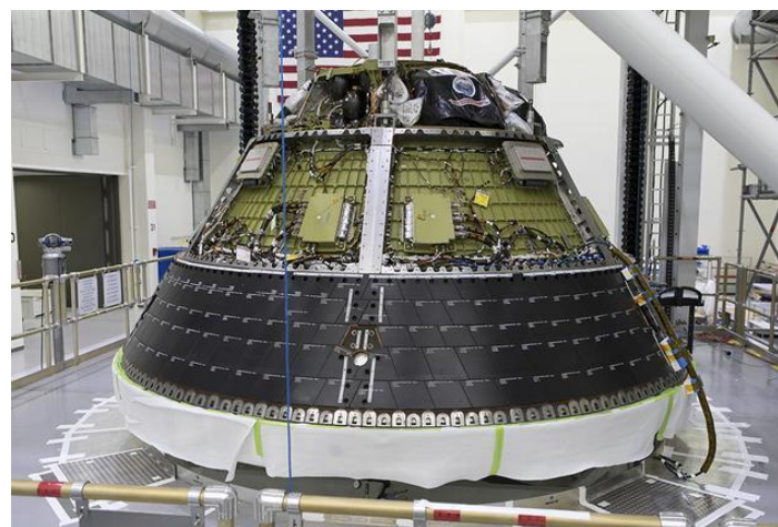
Heat shield back shell panels are prefitted on the Orion Spacecraft
