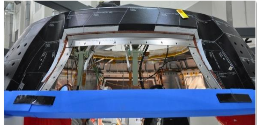
Forward Bay Cover, with Side Panel Removed
