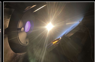
Xe Ion Beam Impinging on Diamond-Like Coating on Kovar Samples in Vacuum Chamber (NASA GRC)
