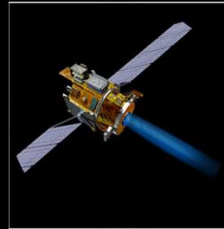
Artist's Drawing of Deep Space I with Solar Electric Propulsion (NASA JPL)
