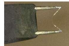
Closeup of Hot Wire probe tip at 50x
