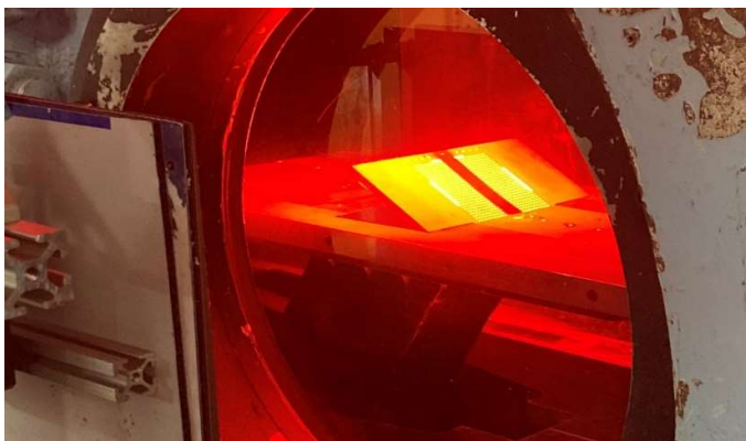
Plate/wedge model under amber-red (616nm) LED lamps
