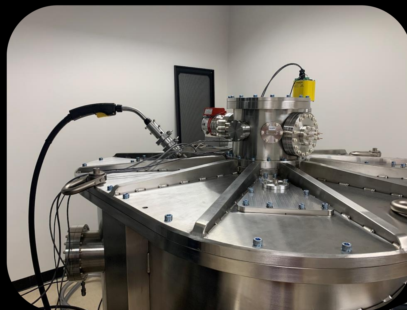
External wire feed on chamber
