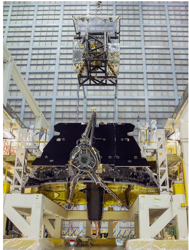
Fig. 2: The ISIM Being Lowered During Installation with the OTE in 2016 [1]
