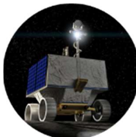
NASA's Volatiles Investigating Polar Exploration Rover, VIPER, is a mobile robot searching for water ice. Credits: NASA Ames/Daniel Rutter
