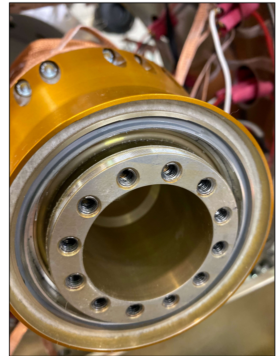
Seals at the LTV actuator outputs removed to check for any simulant inside.
