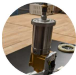
VIPER actuator ready for testing
