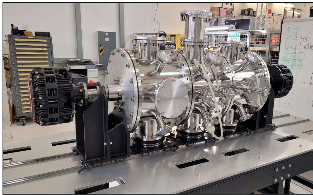
Dusty Vacuum chamber for dynamic seal testing at KSC GMRO Lab 12
