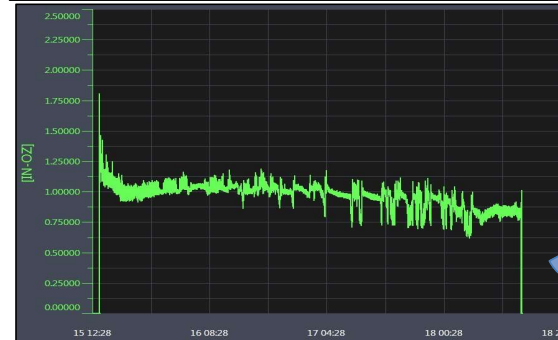
Representative Bearing Torque Evolution Over Time (~1,000,000 cycles)
