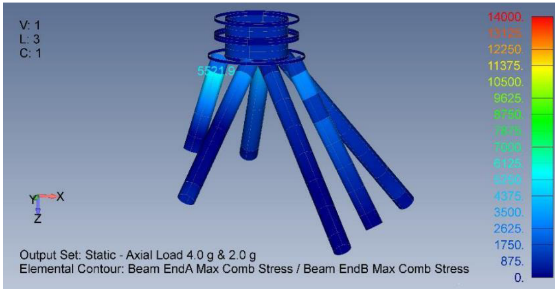
Figure 5.19.—Stress state of the struts supporting the RPS under a 4.0 g axial acceleration and 2.0 g lateral acceleration.
