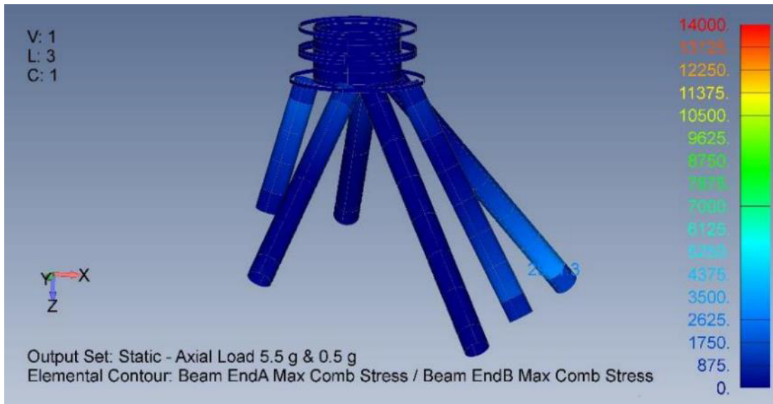
Figure 5.18.—Stress state of the struts supporting the RPS under a 5.5 g axial acceleration and 0.5 g lateral acceleration.
