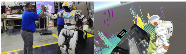
Fig. 10: CSF pipeline commanding Valkyrie in virtual reality. Valkyrie executed commands such as “report listening status,” “set waypoint,” “plan and execute to waypoint,” and “give Lewis a high five,” pictured above.
