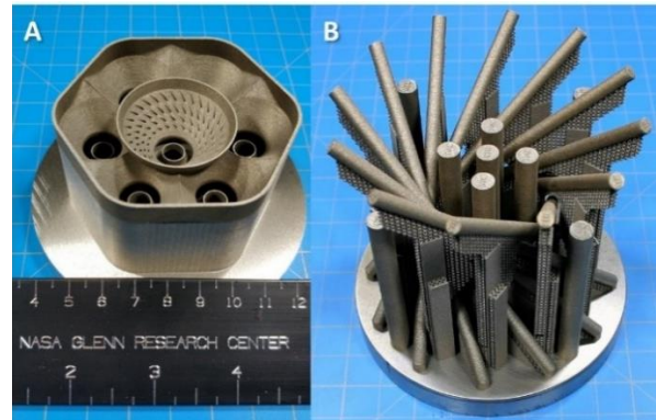
Figure 19. a) An oxide dispersion strengthened 3D printed combustor dome and (b) complex lattice structures.
