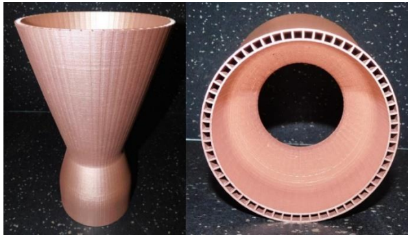
Figure 10. Manufacturing demonstrator chamber using LP-DED green laser and GRCop-42. [Courtesy: RPMI / TRUMPF / NASA].
