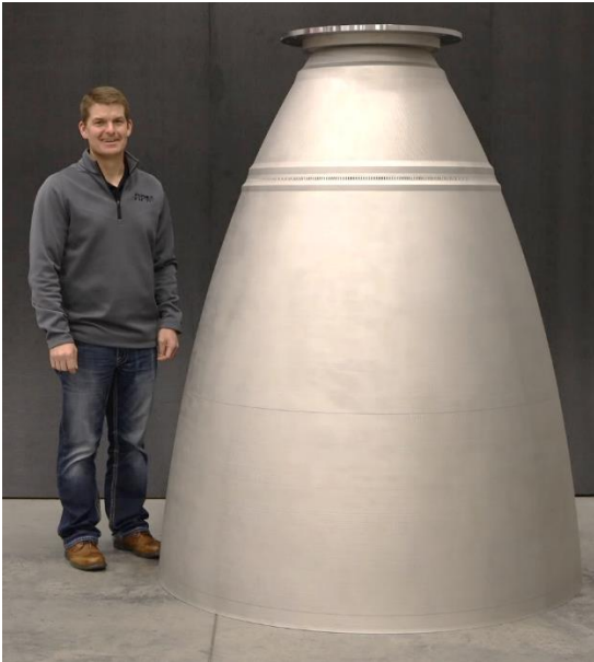
Figure 14. 65% scale RS-25 integral channel LP-DED nozzle using NASA HR-1 (1.52 m dia. x 1.78 m height).
