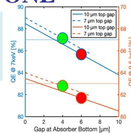
**Fig. 2** Quantum Efficiency Requirements for Athena can be met with trapezoidal shaped absorbers and 4 micron gaps between pixels.
