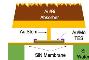
**Fig. 1** A diagram of a GSFC TES pixel. Au/Bi absorber is attached to a Au/Mo TES which is suspended by SiN membrane. The absorber has a trapezoidal shape and a rough surface. A thin Au capping layer is added to improve reflectance at 1-20  $\mu\text{m}$  wavelength range.
