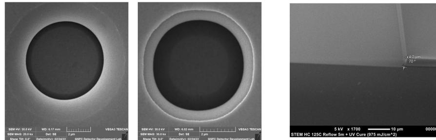
To tune the thermal conductance of the device and the effect on the normal-to-superconducting transition shape, the stems need to be small diameter and can have a weak bottle-neck connection to the substrate. A funnel shape of the stem using a proximity exposed photoresist mold has been developed to improve the strength of the connections.
