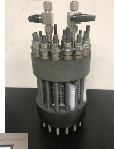
Cell Stack 1 being prepared for vacuum testing
