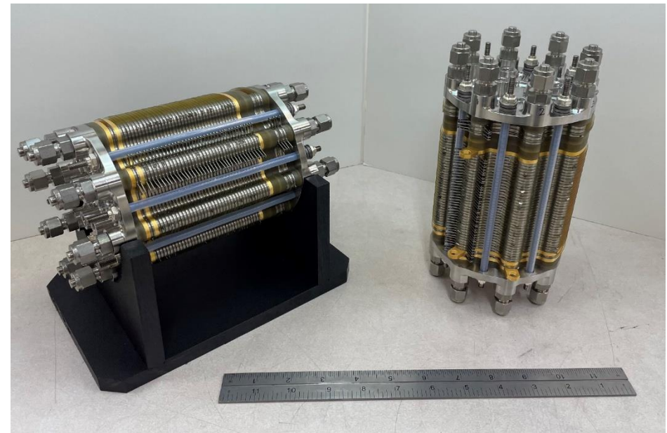
Fuel Cell Stacks 1 and 2
