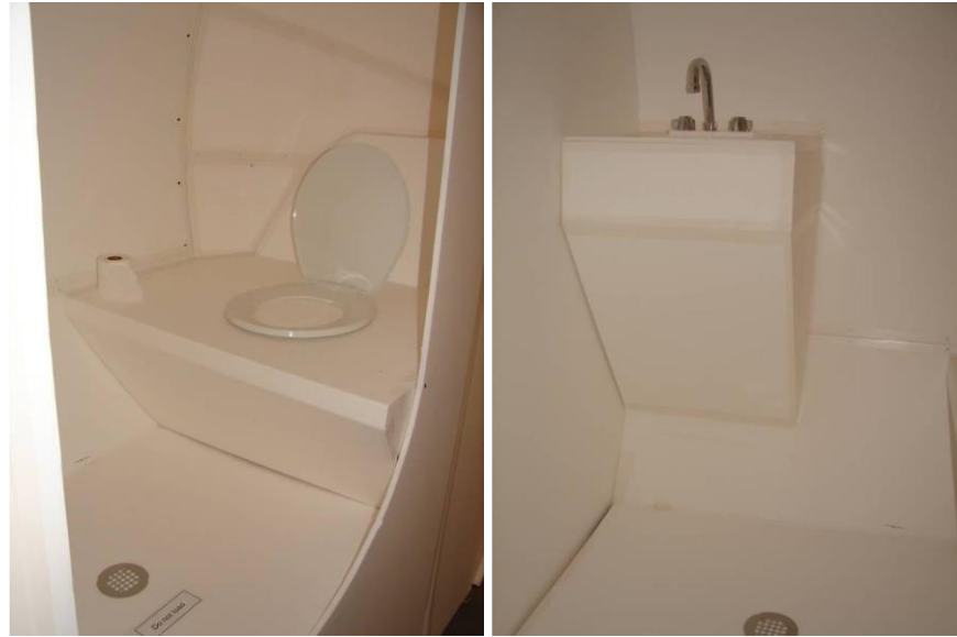
Fig. 19 Waste Containment System
