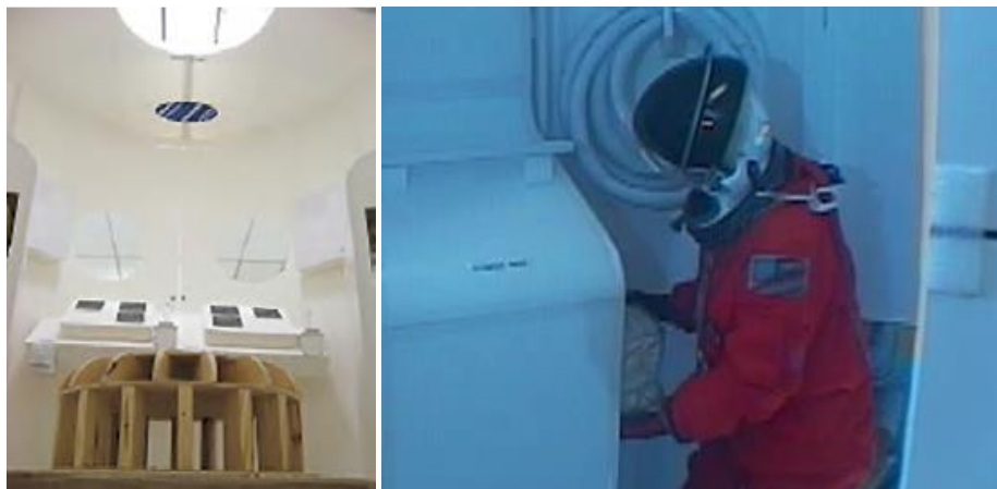
Fig. 12 Ascent Cabin Mockup (left), Subject in ACES Suit Accesses Ascent Cabin Rock Box Stowage Area (right)
