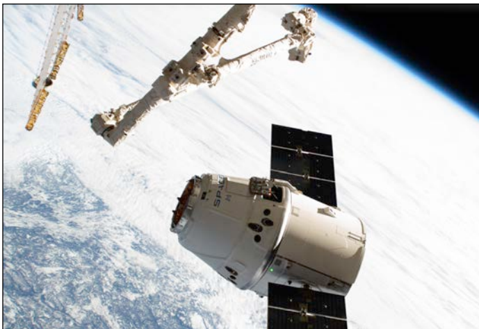
Figure 3. The SpaceX Dragon capsule flown on the Commercial Resupply Mission 17 (CRS-17). The conical capsule's lateral surface is SPAM TPS material. Credit: NASA photo #iss059e043284
