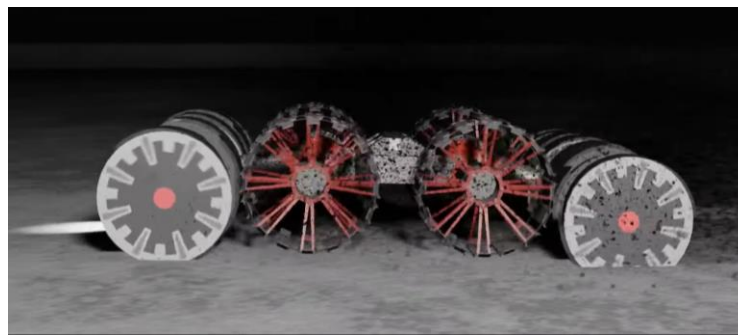
Fig. 4 Redwire's Lunar Regolith Excavator.
