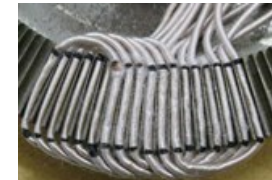
LP Conventional Axial Flux Stator w/Litz Copper Wire Windings
