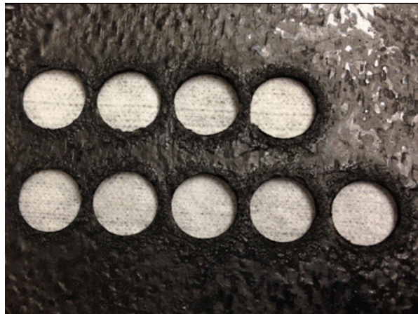
SEM specimens cut with different laser power/speeds
