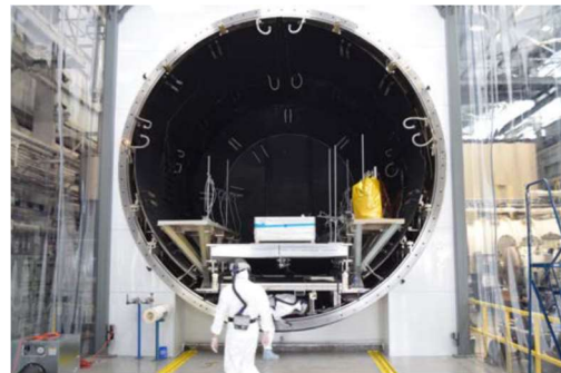
Figure 2. LSS Chamber with Regolith Bed Visible
