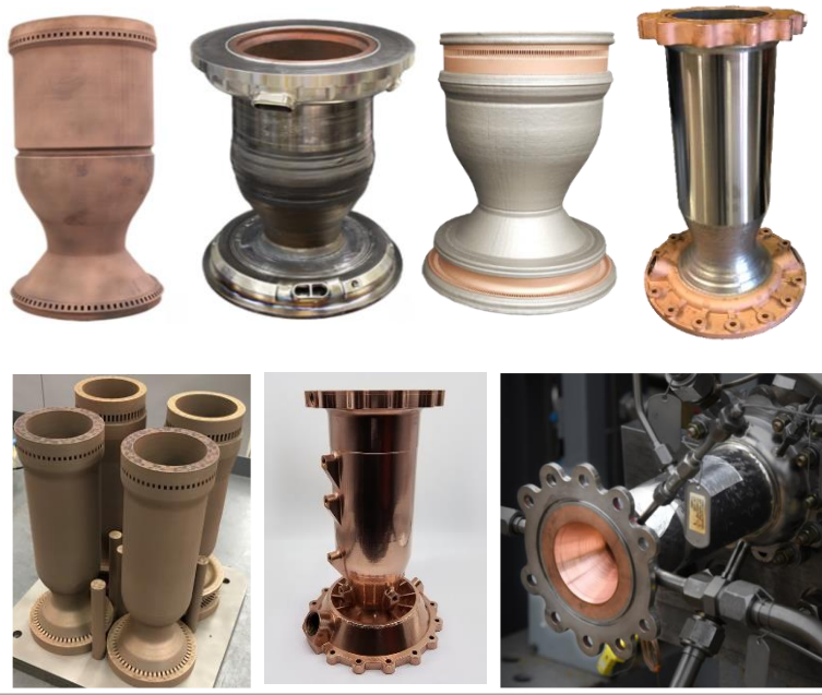
Laser Powder Bed Fusion (L-PBF) Copper Alloys combined with other AM processes to provide bimetalllic
