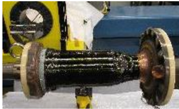
Completed Hoop Layer
