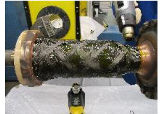
Completed Helical Layer
