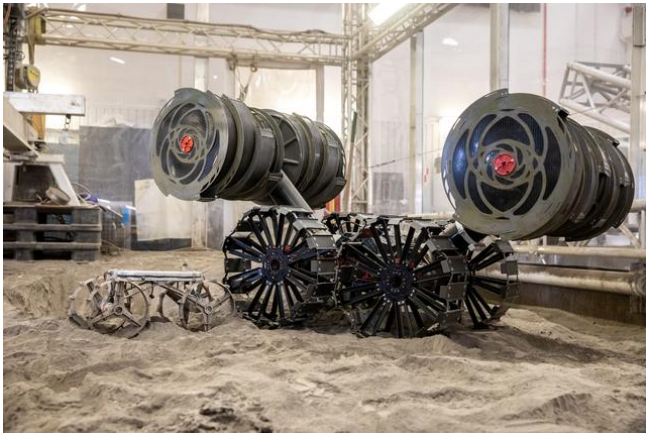
Fig. 3: RASSOR 2.0 in the ‘Big Bin’ at NASA’s Kennedy Space Granular Mechanics & Regolith Operations Laboratory. Here, sensor data was gathered to inform the modeling of our simulation.
