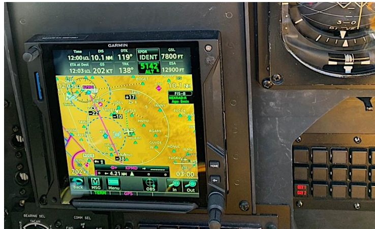
Fig. 12 The NASA ER-2 airplane equipped with Automatic Dependent Surveillance-Broadcast In device (photograph courtesy NASA / James G. Nelson).
