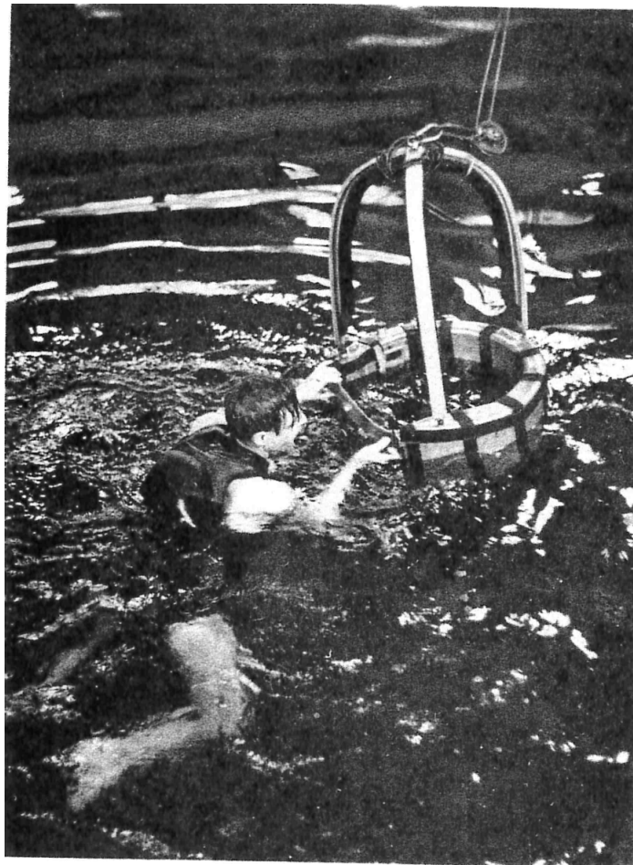
Fig. 36: Lift cage for Fa 223 - sea rescue aircraft
