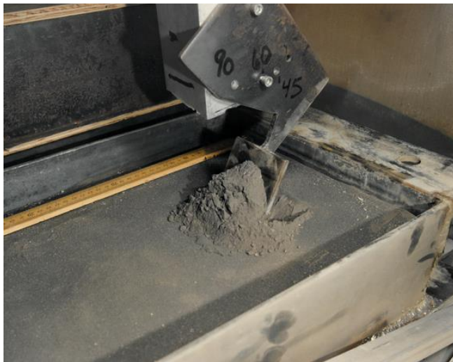
Figure 12. A 1/6-g lunar soil simulant excavation experiment aboard NASA’s KC-135 yielded lower excavation forces of compacted lunar regolith simulant required in lunar gravity compared to Earth gravity and concluded that “A complex relationship exists between gravity and excavation forces” [5]
