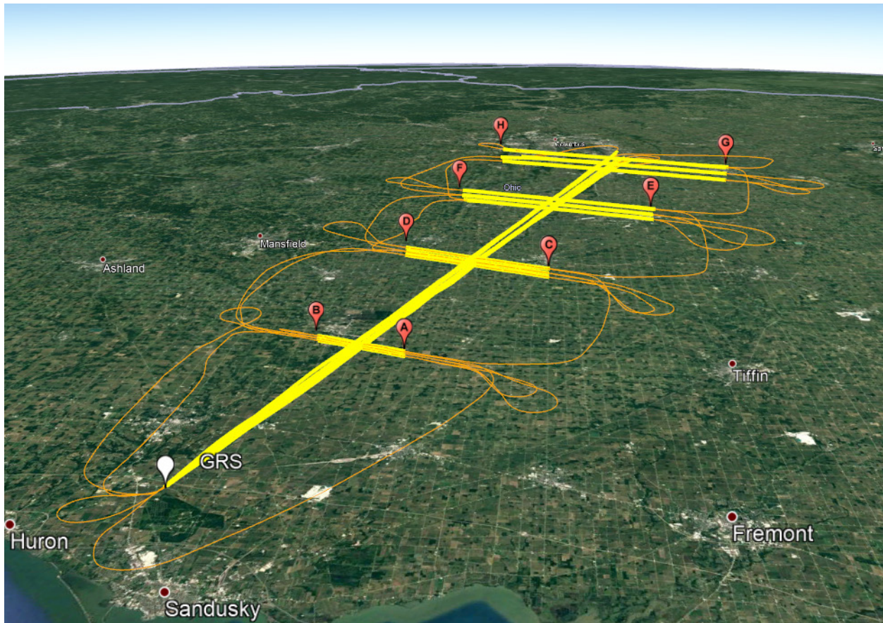
Figure 31.—Perspective view of flightpath over flat terrain highlighting data capture segments, October 8, 2019. Image ©2018 GoogleEarth.
