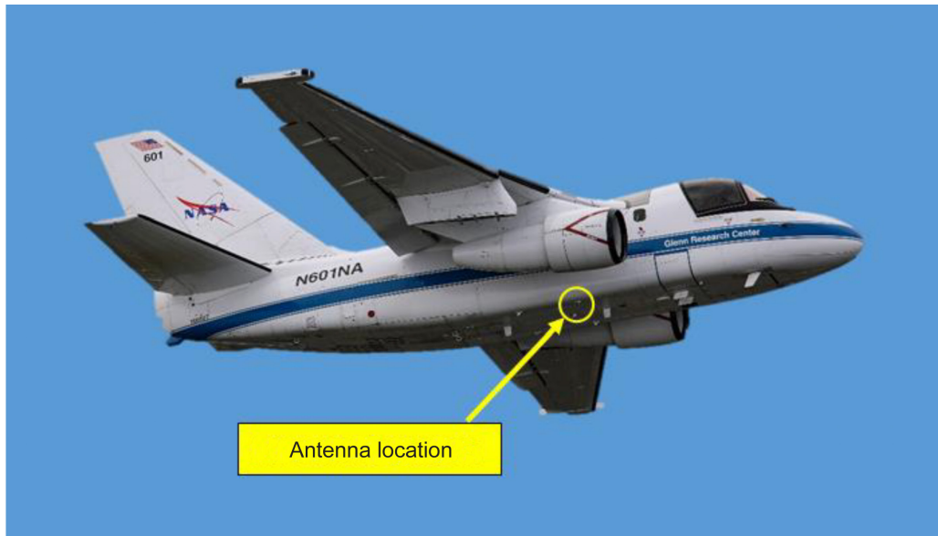
Figure 12.—NASA S-3B Viking test aircraft showing antenna mounting location.
