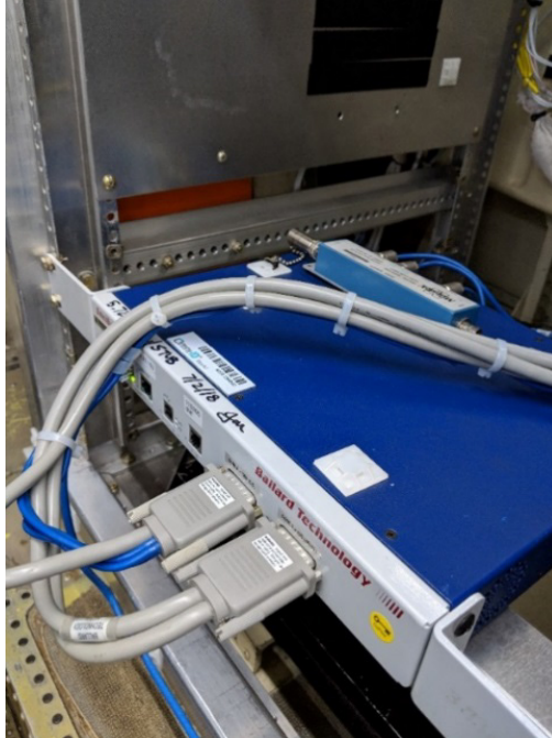
Figure 15.—Aircraft telemetry interface.
