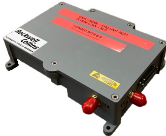
Figure 1.—Control and Non-Payload Communications (CNPC) C-band prototype radio (CNPC–5000E).
