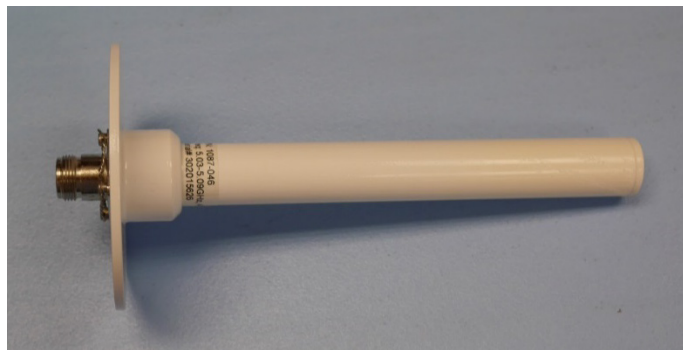
Figure 23.—Ground station C-band omnidirectional antenna.
