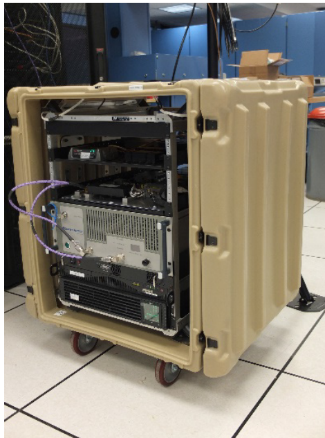
Figure 7.—Ground radio system (GRS) transportable equipment.
