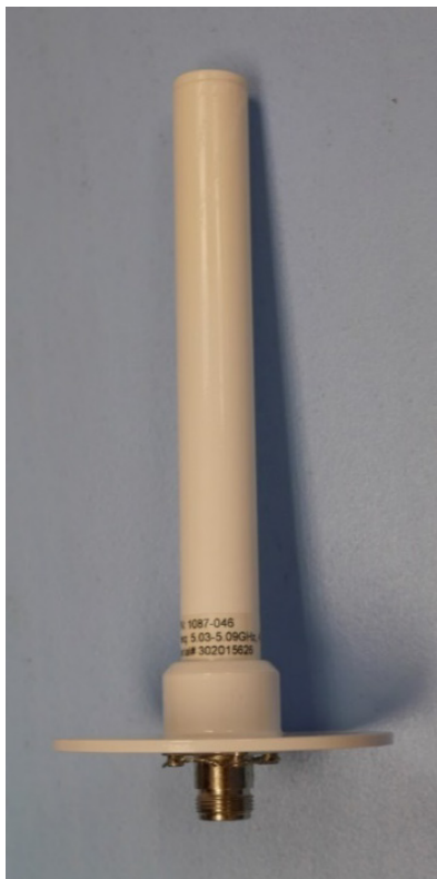
Figure 13.—Ground station C-band omnidirectional antenna.
