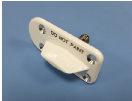
Figure 4.—C-band aircraft antenna.
