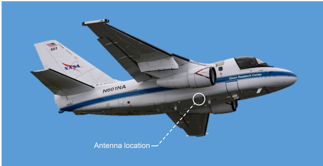
Figure 3.—NASA S-3B Viking test aircraft showing antenna mounting location.
