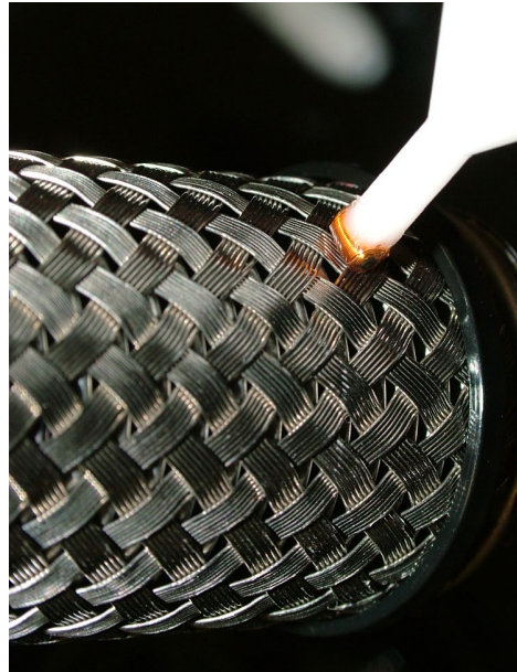
Radiator Flex Hose Cracking
