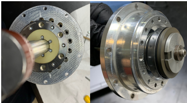
Figure 14. The input half of the SWG actuator
