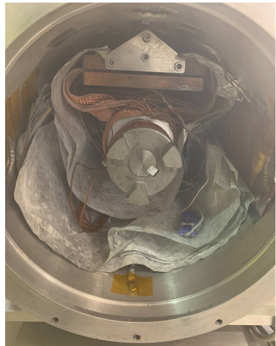
Figure 20. A CSG-20 SWG set up for a cold test
