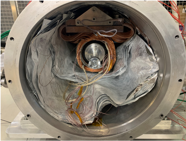
Figure 21. An LSI 75-12 set up for a cold test
