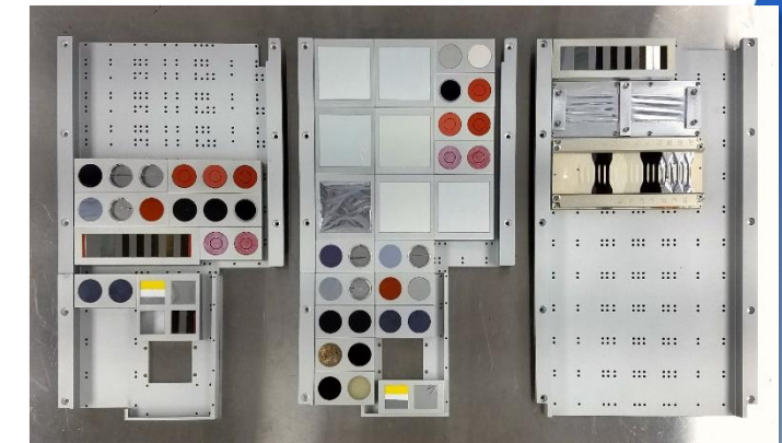
Pre-flight photograph of the PCE-4 flight samples in the M13 Z2 (left) and M13 W1 decks (center & right)
