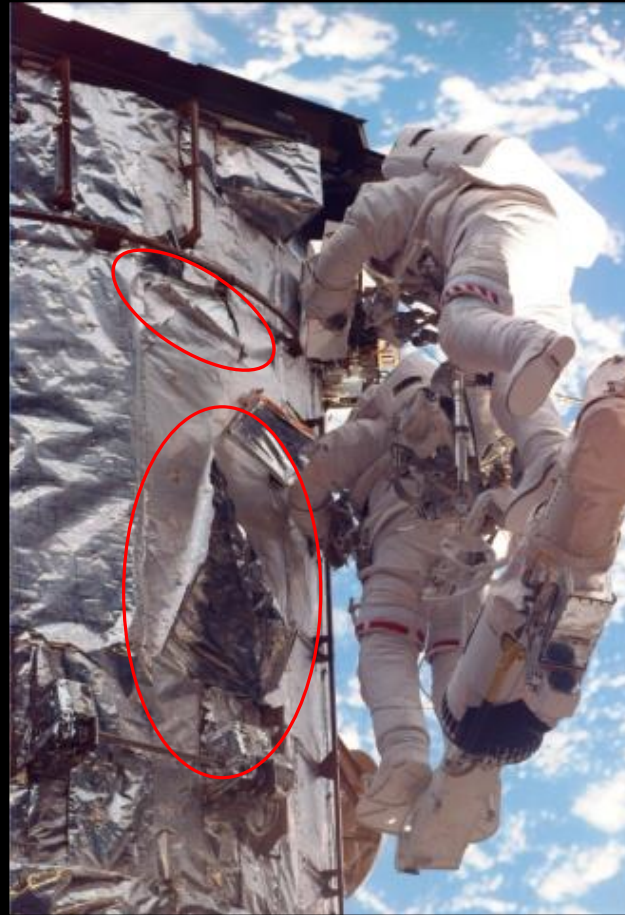
Servicing Mission 2 (SM2) 6.8 years of space exposure
