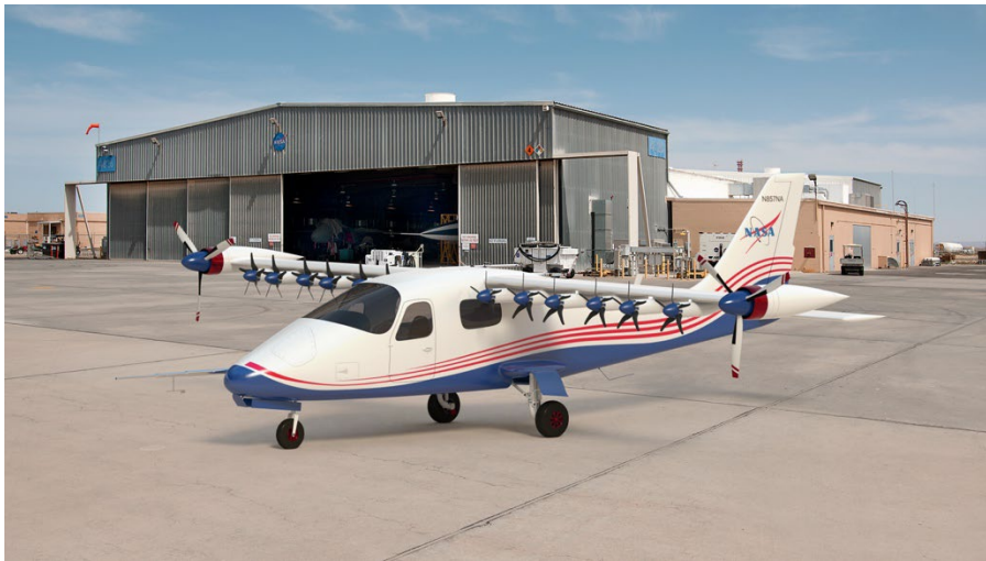
Figure 3. Artist's Rendition of the NASA X-57 Mod IV Distributed Electric Propulsion Flight Demonstrator
