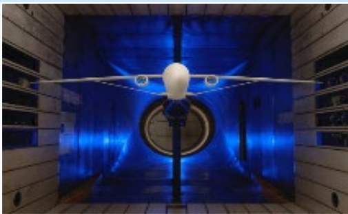
Transonic Truss-Braced Wing 5-10% fuel burn benefit
