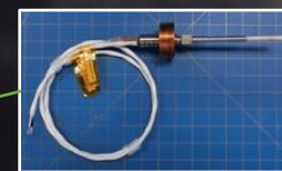
Radiometer sub-assembly prior to installation into heat shield
