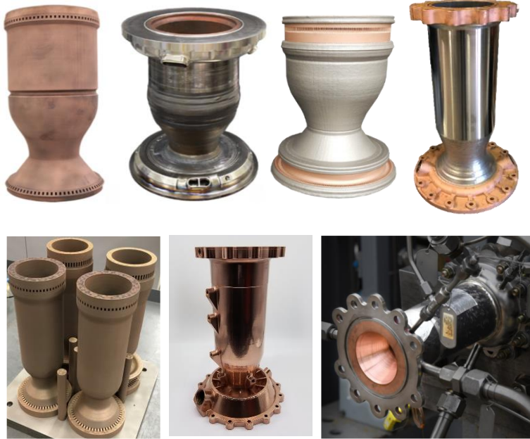
Laser Powder Bed Fusion (L-PBF) Copper Alloys combined with other AM processes to provide bimetallic
