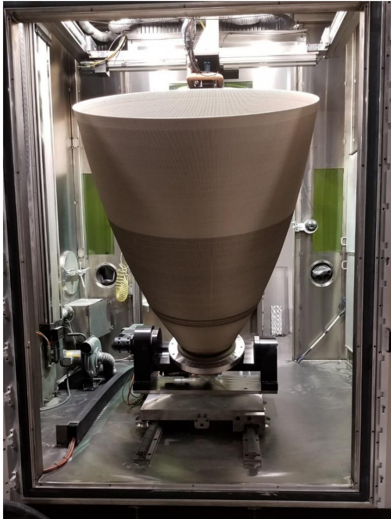
1.52 m diameter and 1.78 m height with integral channels 90 day deposition
