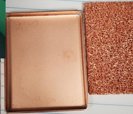
Cu-Mo-Cu enclosure for TMS system testing
