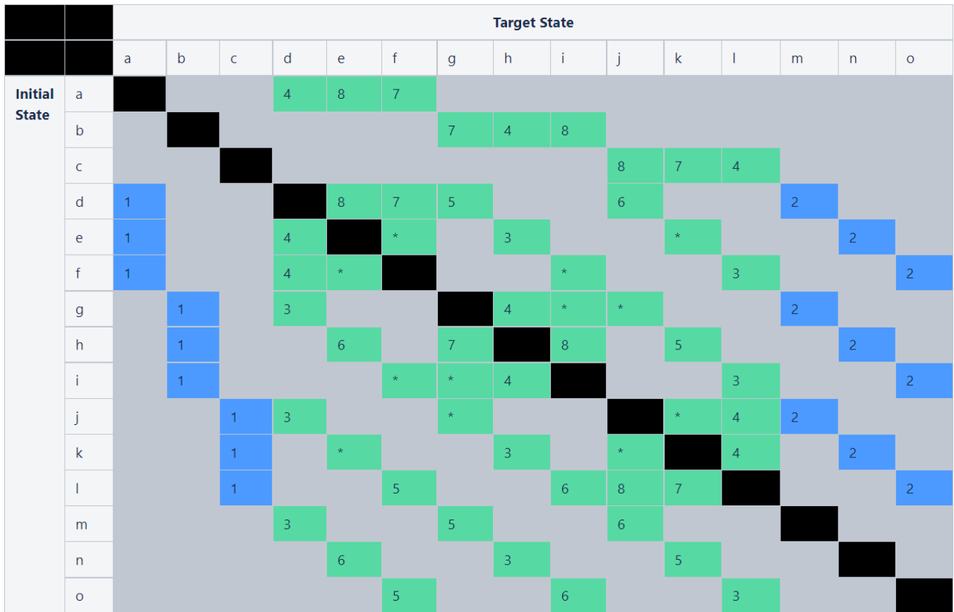
Figure 9. MMIC-I's reconfiguration map. It determines if it's possible to transition from an initial state (column on the left) to a target state (row above) using a single primitive. A colored-background cell filled with a number identifies a possible transition through that specific primitive number.
