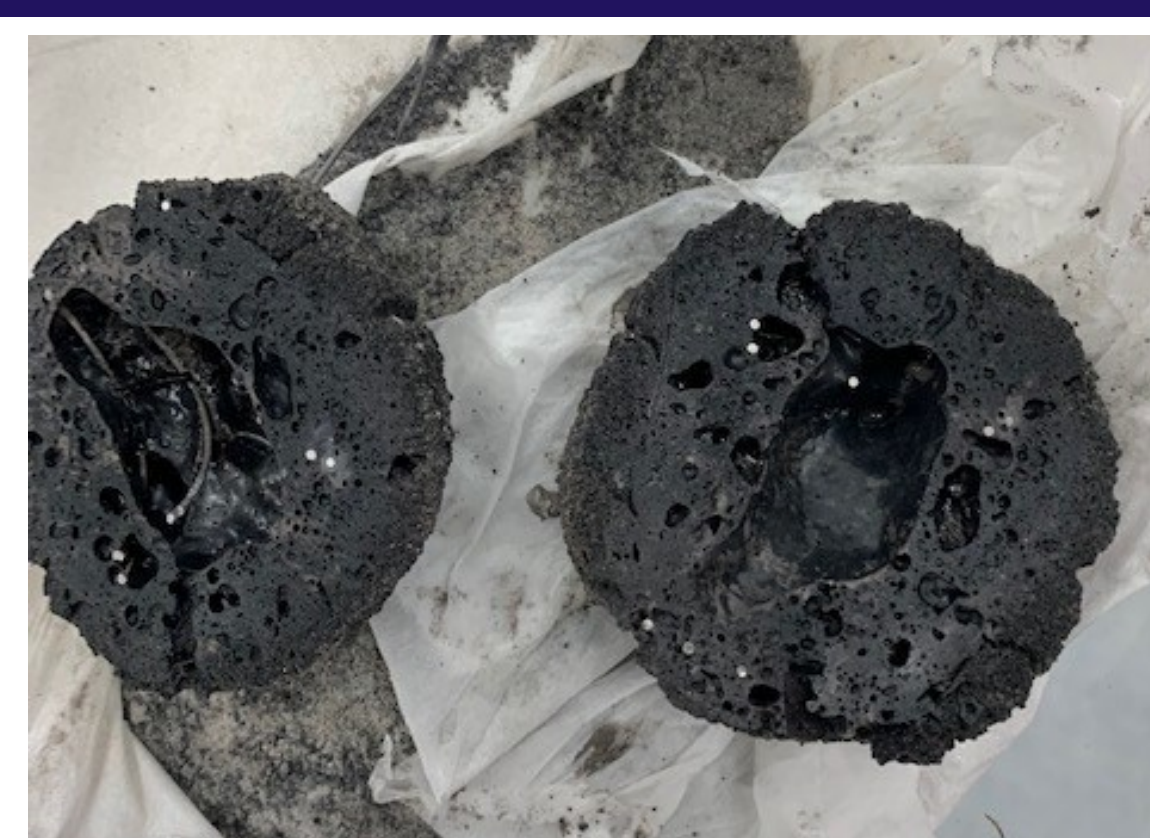
Hardened sphere split in half with diamond saw to show void formation consistent with atmospheric testing. Cross-sectional view.
