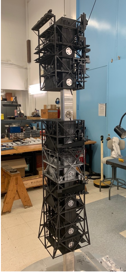
Fig. 8 Photograph of the ML-2 tiers showing Mini-45 load cells.
