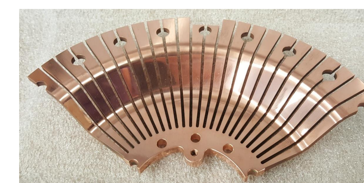
Full-scale Cu thermal bridge (piece 1 of 3)
