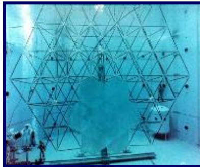
Figure 4. Astronaut assembled 14-m precision segmented reflector truss.
