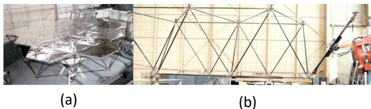
Figure 5. Truss structures assembled in the ASAL: (a) a primary reflector and (b) the backbone truss.
