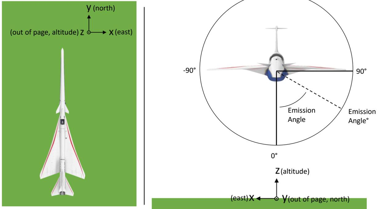
Figure 3-9 RAYTRACING coordinate axis definition.
