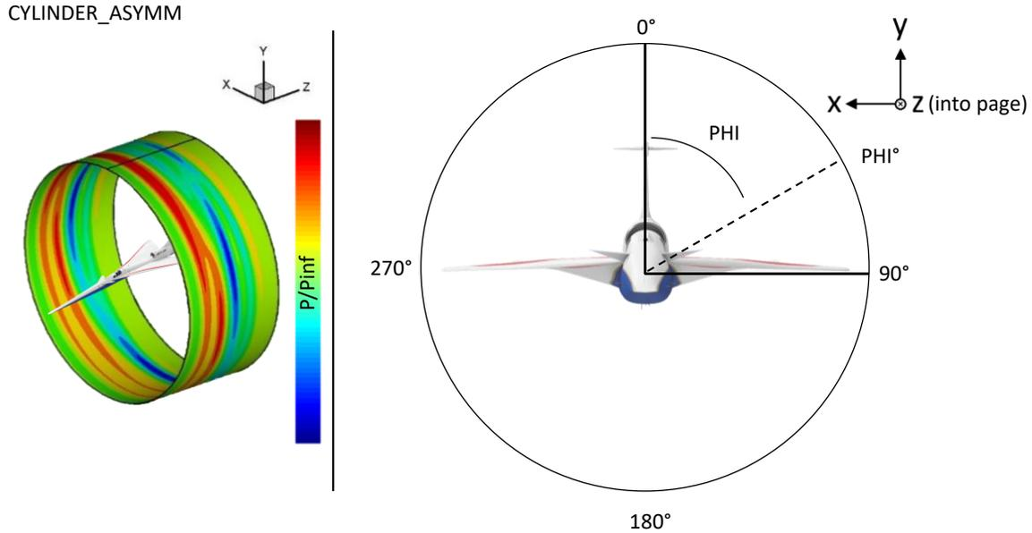
Figure 3-17 CYLINDER\_ASYMM coordinate axis definition.
