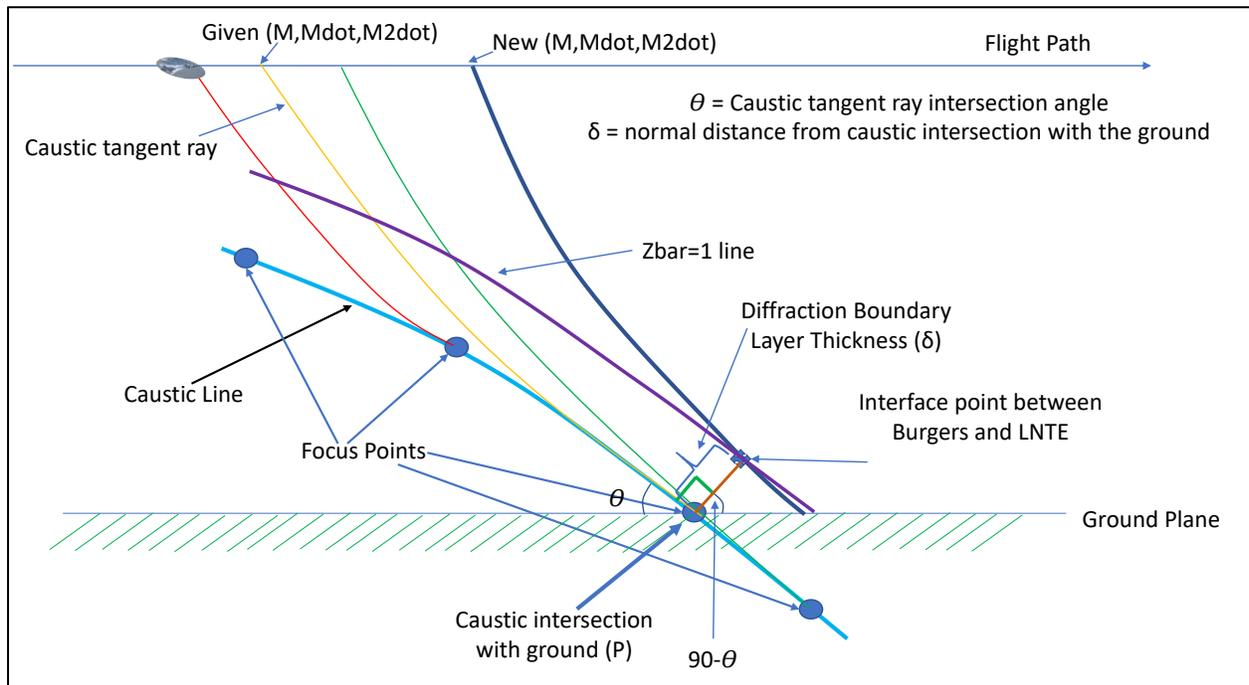
Figure 5-1 Focus delta ray geometry.<sup>13</sup>
