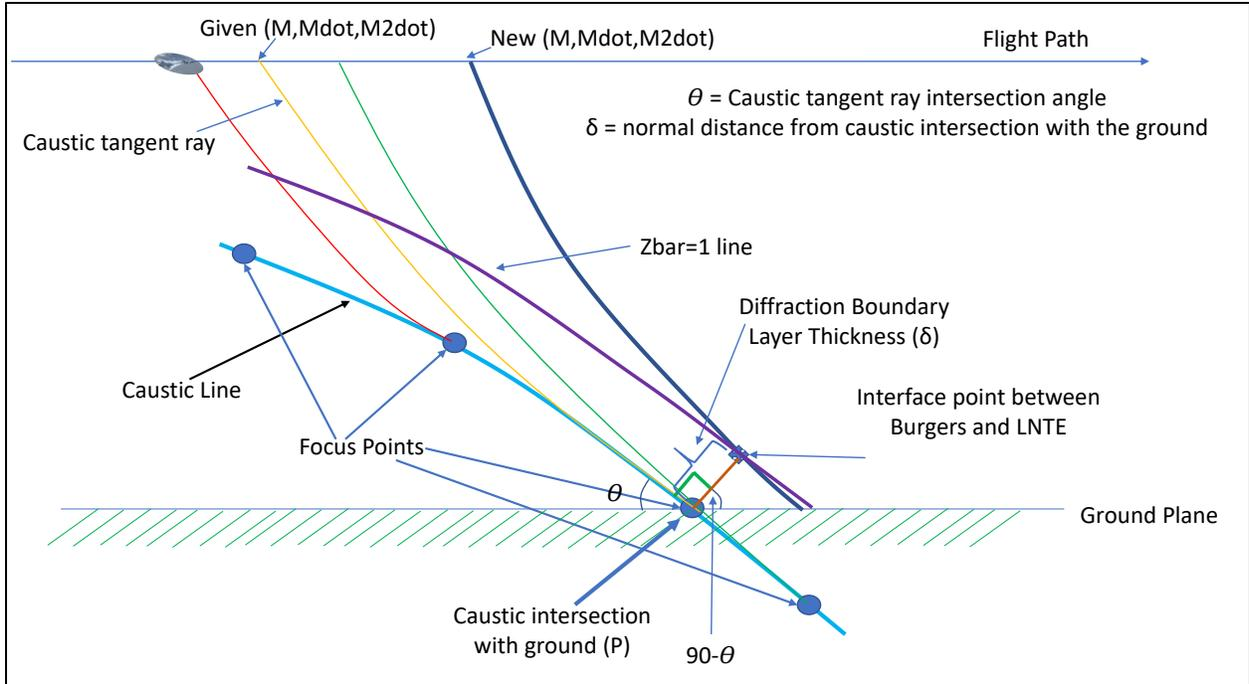
Figure B-55 Focus delta ray geometry.<sup>21</sup>
