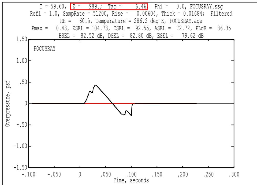
Figure B-69 PCBurg focus delta ray propagation termination at Burgers-LNTE interface altitude and  $T_{ac} = TADVANCE$ .
