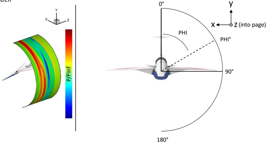
Figure 3-13 CYLINDER coordinate axis definition.
