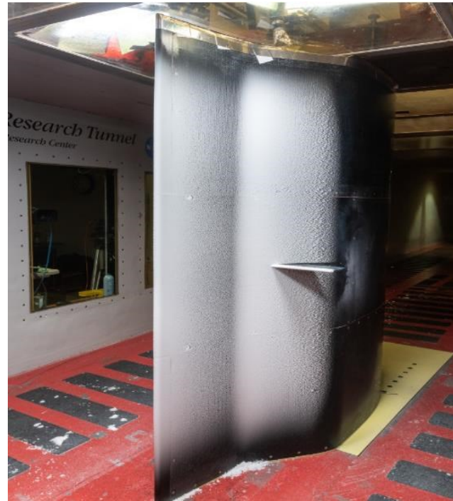
Supercooled liquid ice accretion on SIDRM
