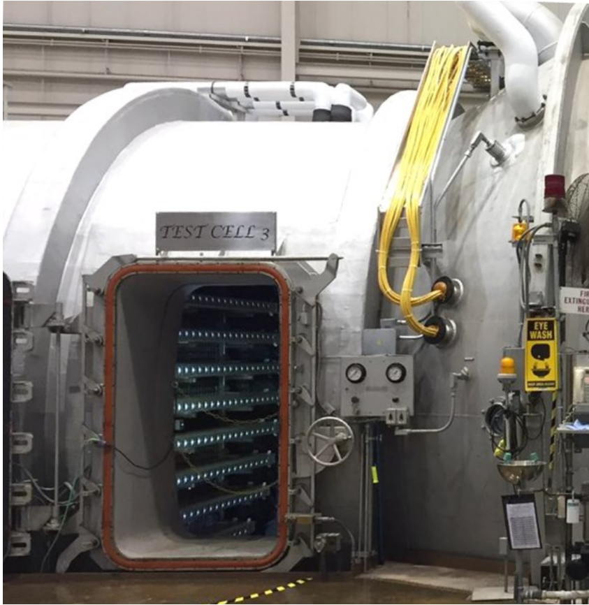
Plenum with Spray Bars, \Phi = 18\text{-ft}
