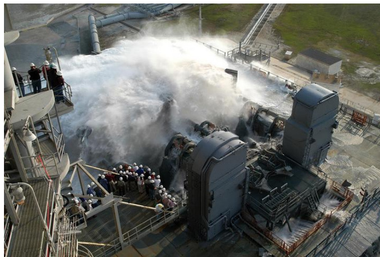
Photographs of a test of the NASA Kennedy Space Center (KSC) water deluge system which is used to suppress the immense sound pressure levels felt by the vehicle and surrounding structures during ignition.
