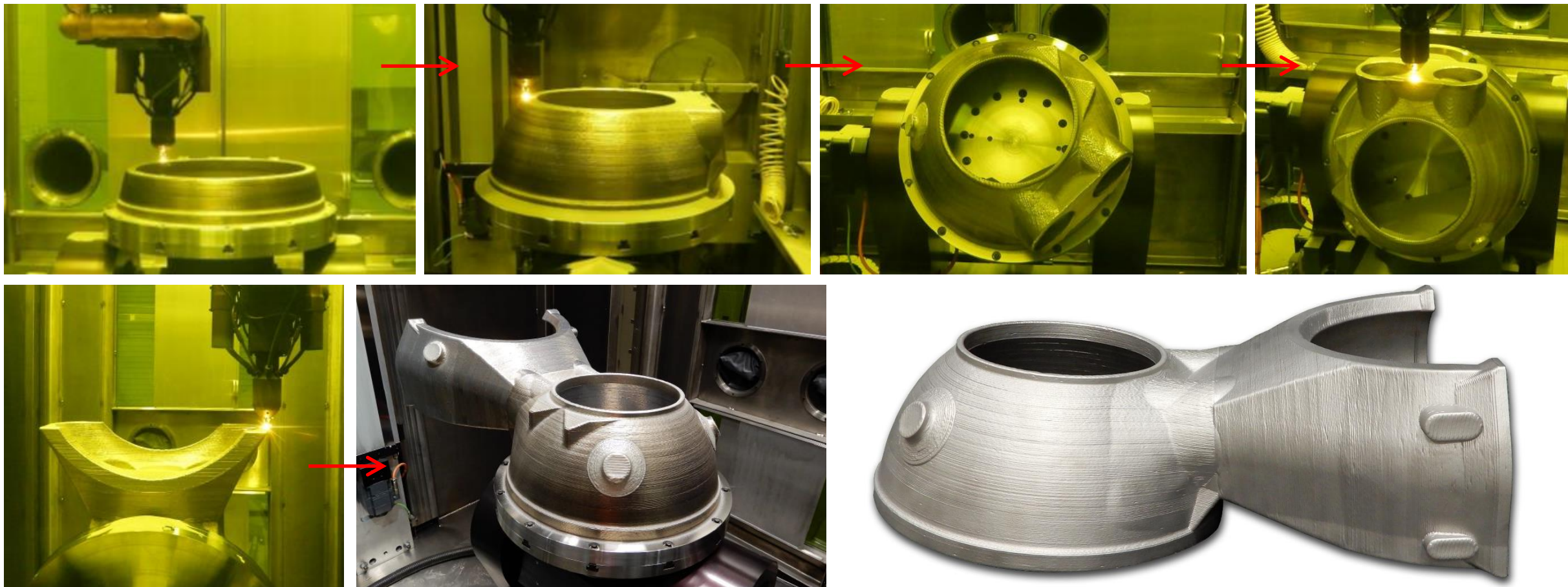
RS25 Powerhead demonstrator using LP-DED under NASA SLS Artemis Program (Courtesy: RPMI)
