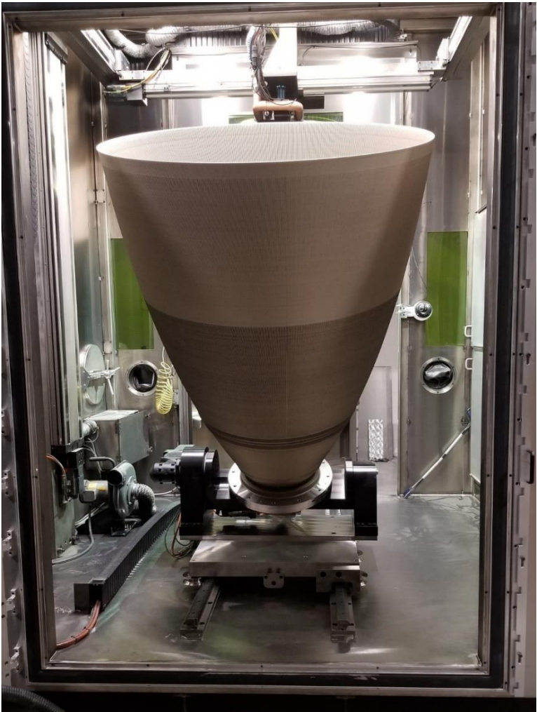
60" (1.52 m) diameter and 70" (1.78 m) height; thin-wall with integral channels 90 day deposition
