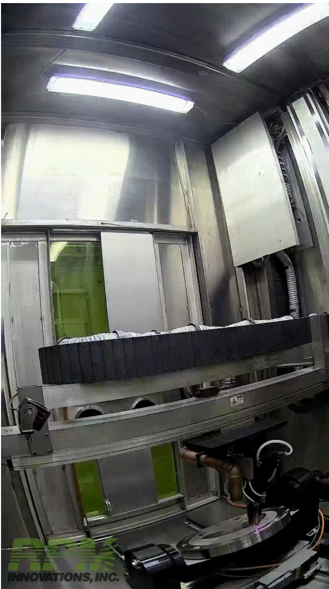
60" (1.52 m) diameter and 70" (1.78 m) height; thin-wall with integral channels 90 day deposition
