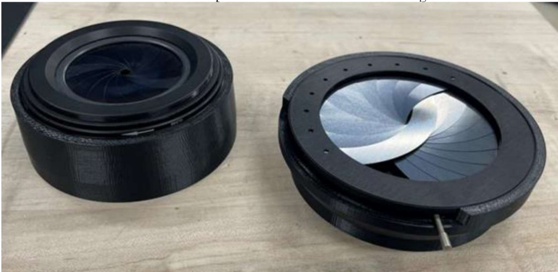
Fig. 6 Iris mechanisms with 3D-printed adapters.
