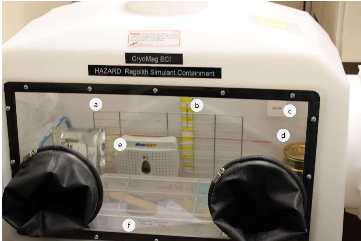
Fig. 3 The DELTA glovebox used for testing, loaded with the necessary equipment: (a) wire rack, (b) paper ruler, (c) temperature/humidity remote control, (d) sieve stack, (e) rechargeable desiccant, and (f) regolith simulant discard box.
