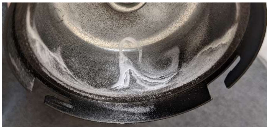
Fig. 9 Dust adhered to filter housing.
