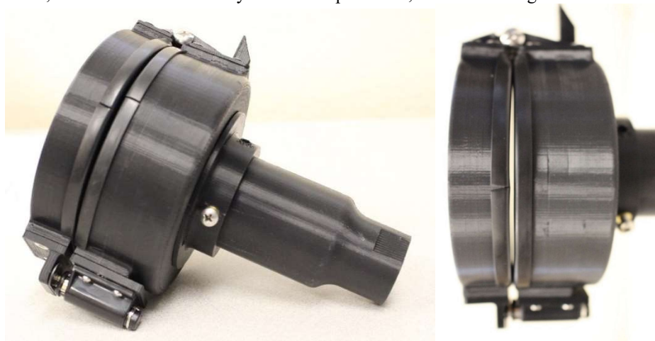
Fig. 15 The 3D printed cap-and-sleeve DMS prototype (left), and a close-up of the deficient gap when closed (right).
