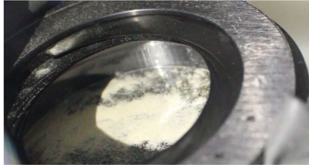
Fig. 14 Dust intrusion through blackout iris after multiple actuations.
