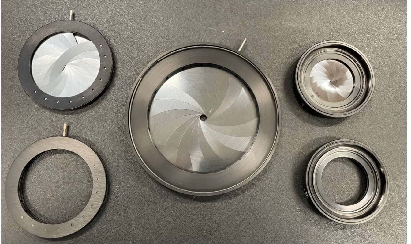
Fig. 2 Iris mechanisms, from left to right, lever-actuated 75-mm blackout aperture, lever-actuated 120-mm aperture, and ring-actuated 50-mm aperture.
