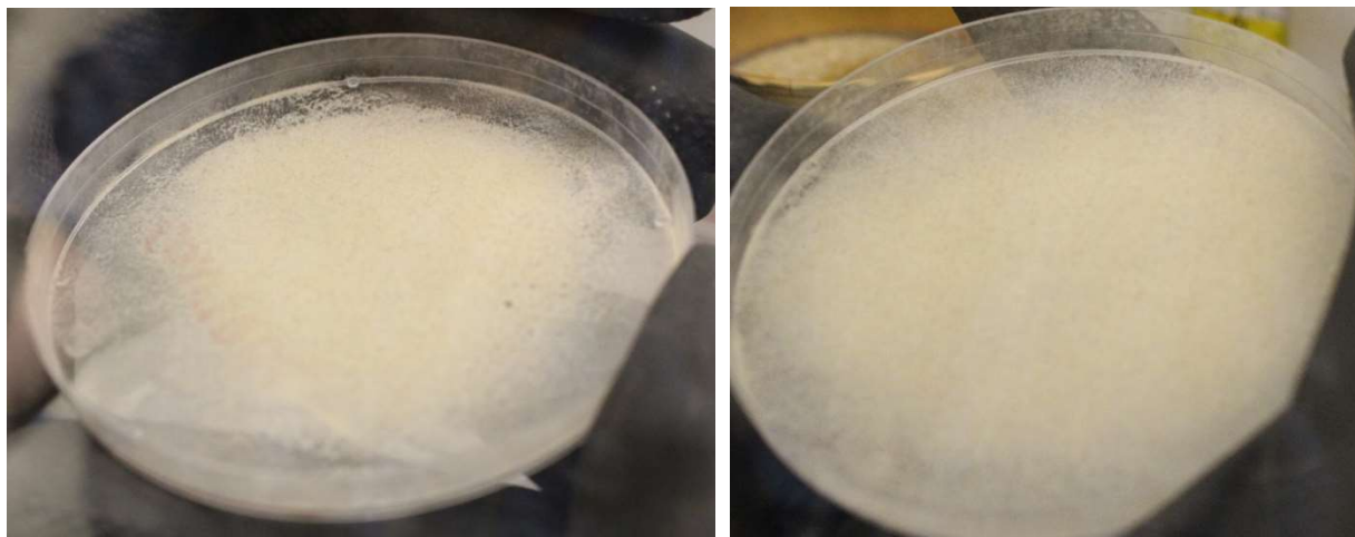
Fig. 10 Dust dispersion evaluation initial attempt (left), and more evenly dispersed (right).
