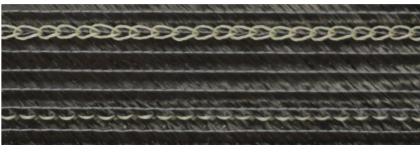
a) 5-mm stitch length conventional seam
