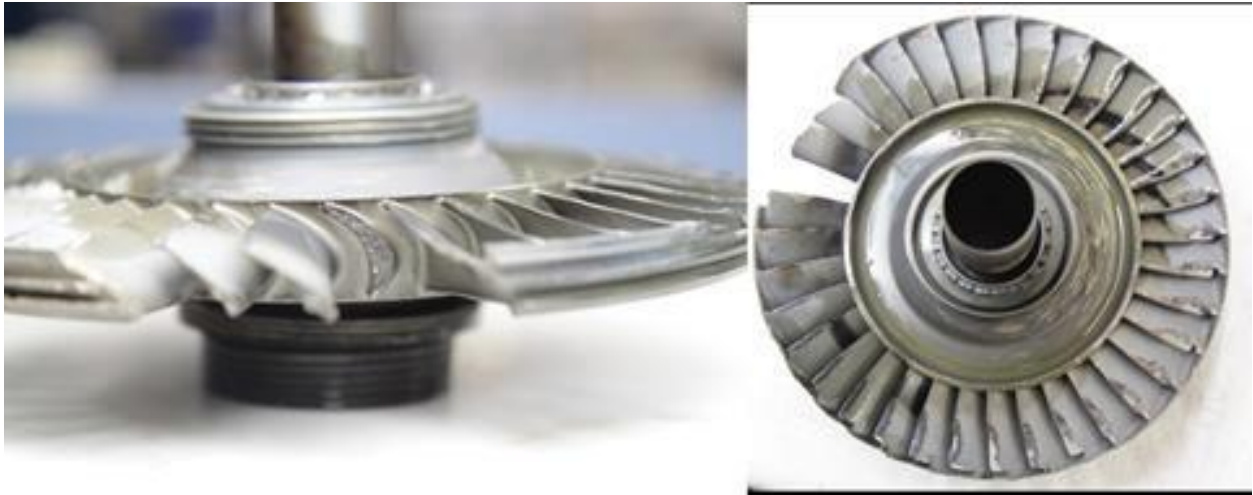
Figure 1. Blisk with blade failure
