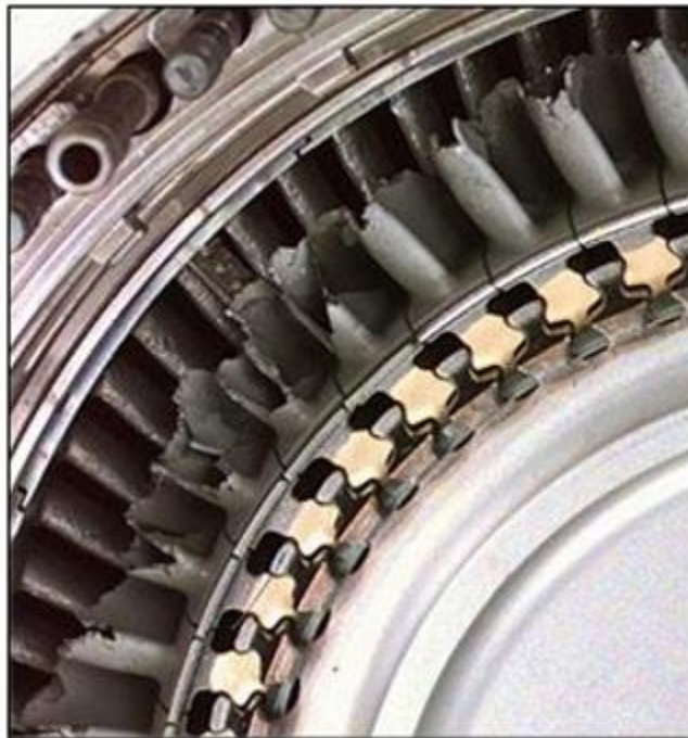
Figure 2. Inserted bladed-disk with blade failures
