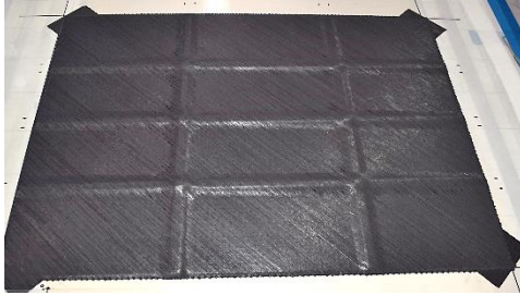
(a) Orthogonal stiffeners replicating traditional spars and ribs (b) Stiffener angle investigation
