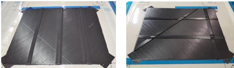
Figure 19. Stiffened panels containing only composite material.
